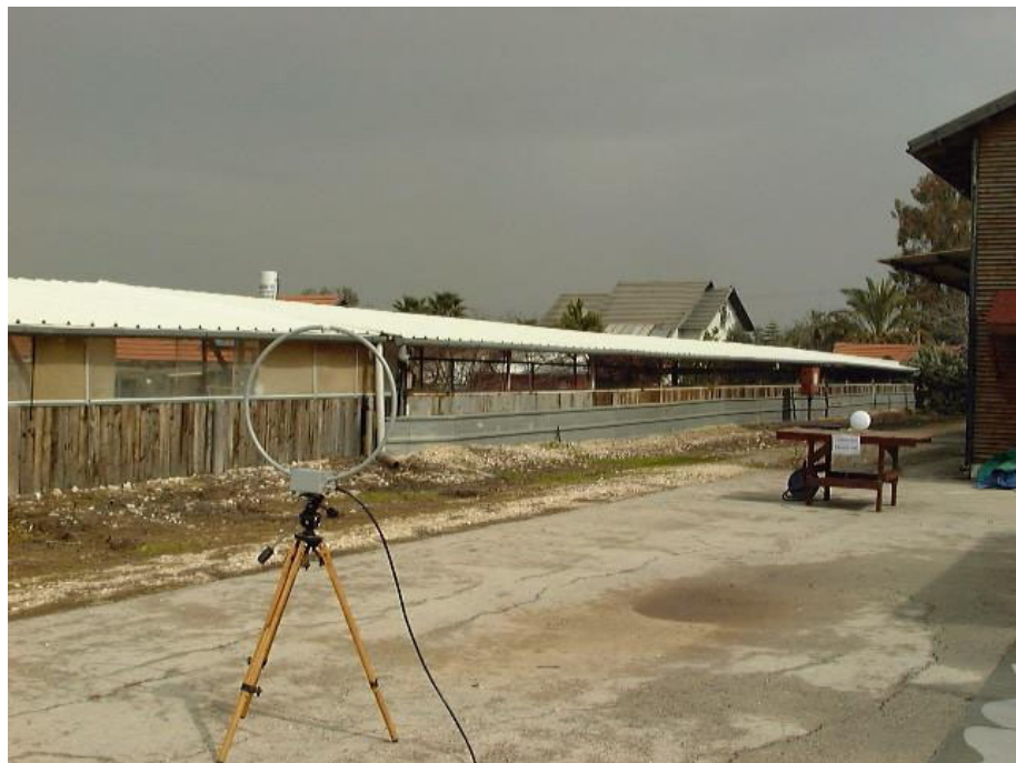
Figure 2. Radiated Emission Test 9 kHz – 30 MHz
