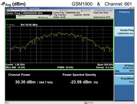
$PAPR (dB) = P_{Pk} (dBm) - P_{Avg} (dBm) = 30.68 dBm - 30.30 dBm = 0.38 dB$
