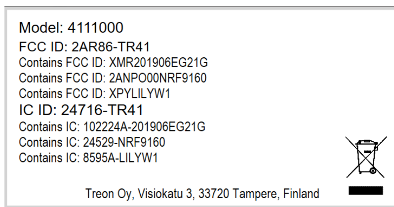
Figure 1. Label example of 4111000 – Size not in scale. Actual label size 2 x 1 inch.
