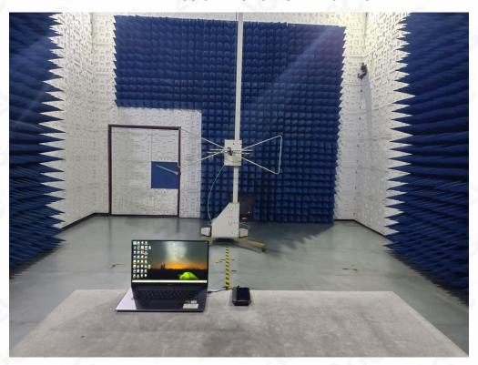
RADIATED EMISSION TEST SETUP ABOVE 1GHz
