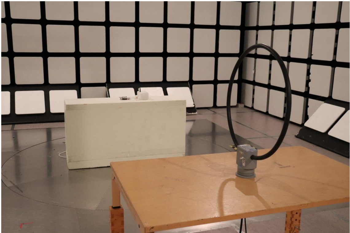
Photograph 6. Radiated Spurious Emissions 9 kHz – 30 MHz
