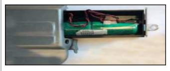
4. The lock should be available for installation about 10 seconds after battery installation.
