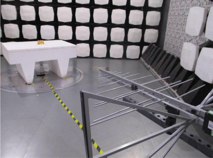
**1.4 Radiated Emissions Test Setup(Above 1GHz)**
