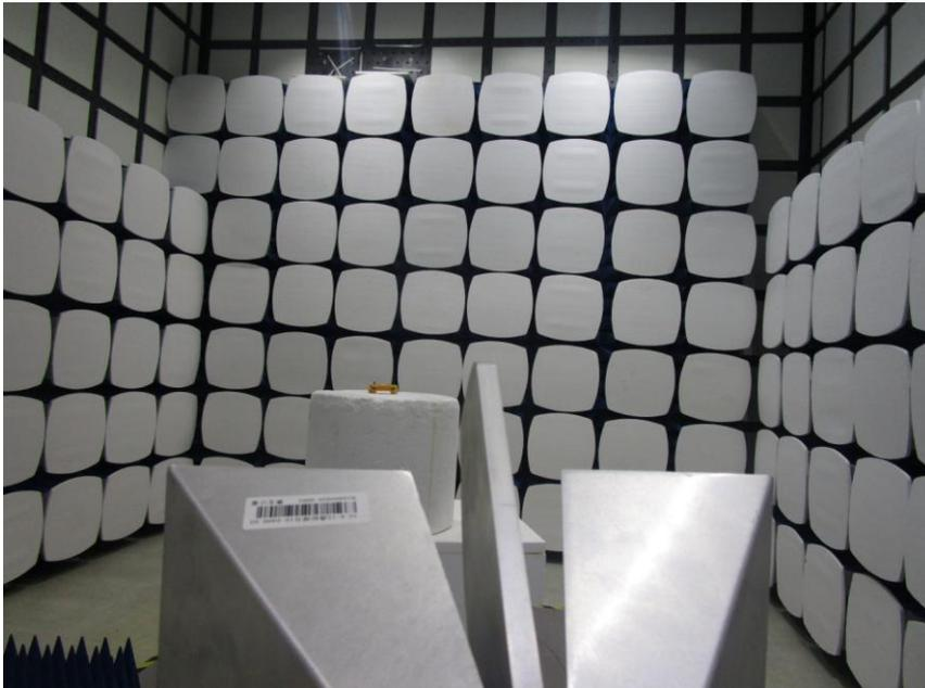
**1.3 Radiated Emissions Test Setup(30MHz~1GHz)**
