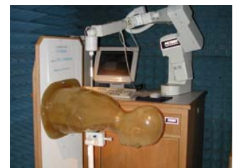
Fig. 1 SAR Test Setup
