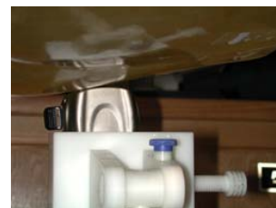
Fig. 10 Hand SAR Test Setup
