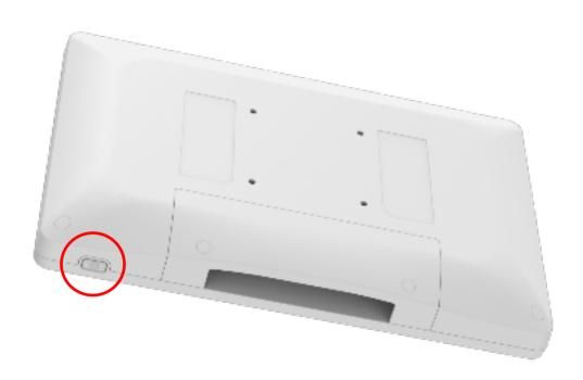
6. VESA 75mm mounting M4 screw holes (10mm x 4 ), use VESA qualified stand or bracket to install
