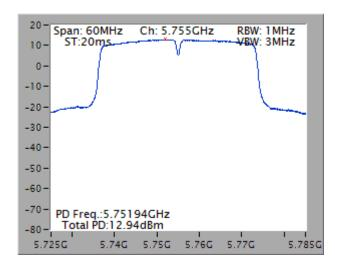
Power Density Plot on Configuration IEEE 802.11ac MCS0/Nss1 VHT80 / Chain 1 + Chain 2 + Chain 3 / 5775 MHz
