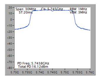
Power Density Plot on Configuration IEEE 802.11ac MCS0/Nss1 VHT20 / Chain 1 + Chain 2 + Chain 3 / 5825 MHz
