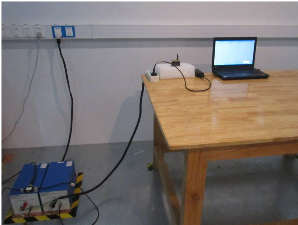
Conducted Emissions Test Setup Front View
