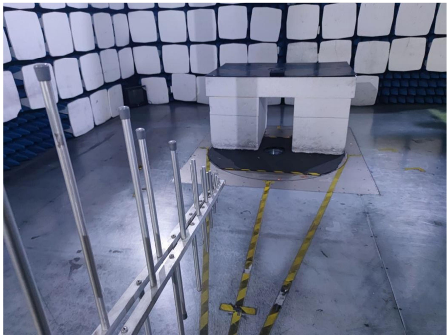
Radiation Emission Test Setup (30MHz to 1GHz)
