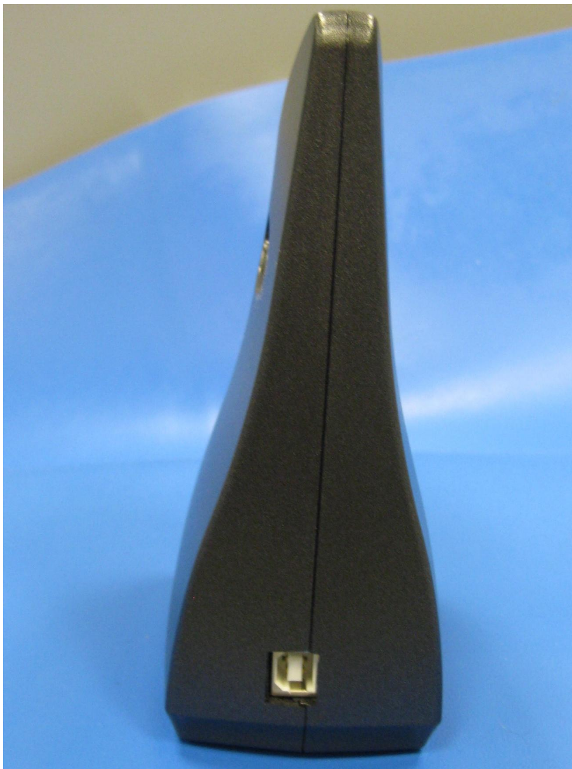
SurfLink Programmer rear view showing USB connector
