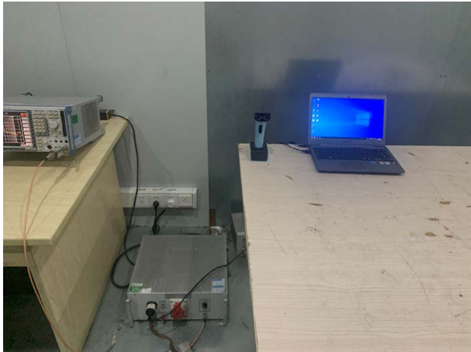
Conducted Emission Test Setup
