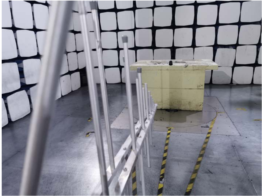
Radiation Emission Test Setup (30MHz to 1GHz)
