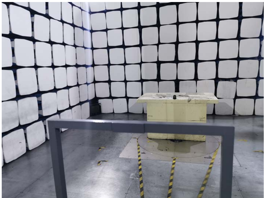
Radiation Emission Test Setup (Below 30MHz)
