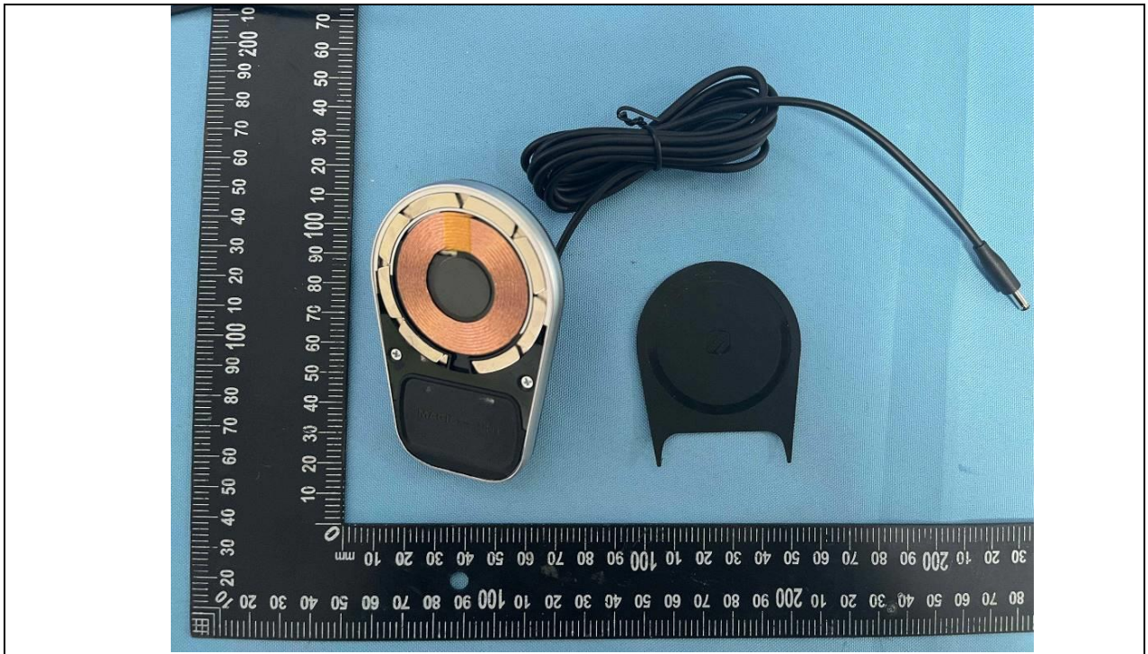
Details of: Wireless charger internal view-2 (Model: MPQ5)
