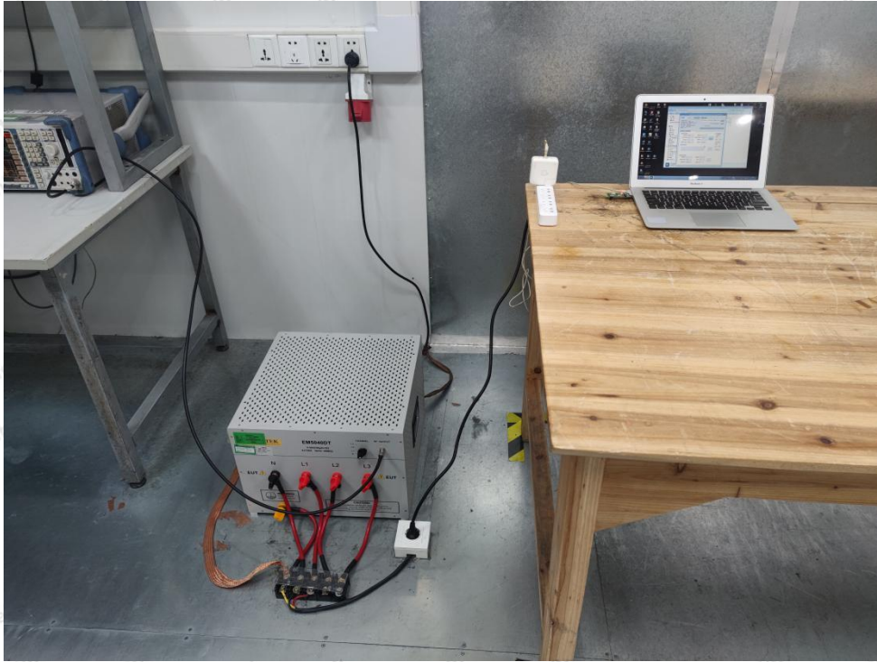
Photo of Conducted Emission Measurement
