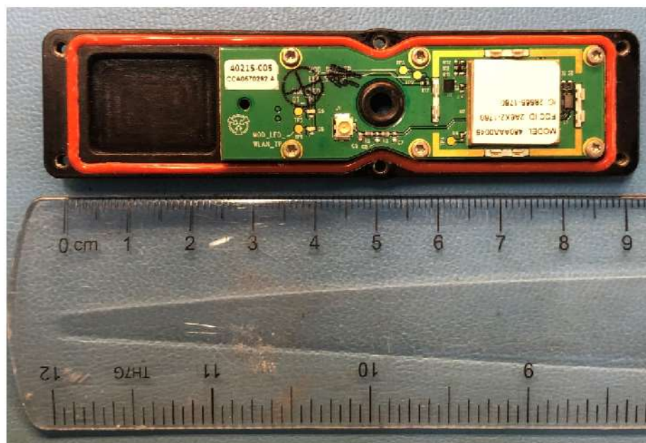
Figure 6: TW-1760 PCB, shield-can removed
