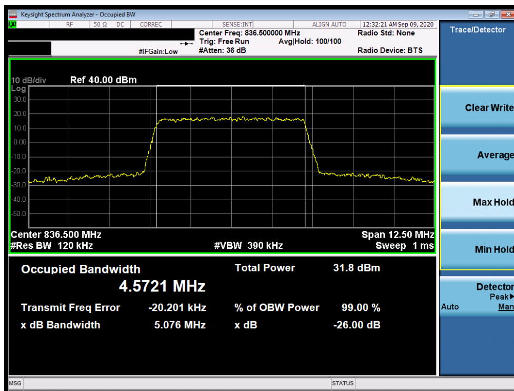
Plot 7-8. Occupied Bandwidth Plot (LTE Band 26/5 - 5MHz 16-QAM - Full RB Configuration)
