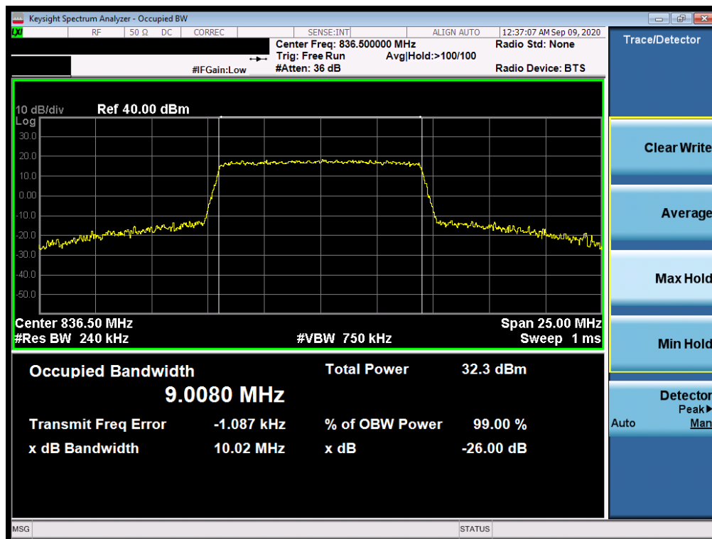
Plot 7-6. Occupied Bandwidth Plot (LTE Band 26/5 - 10MHz 64-QAM - Full RB Configuration)
