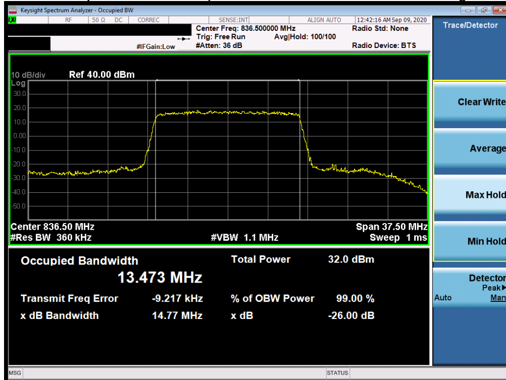
Plot 7-2. Occupied Bandwidth Plot (LTE Band 26 - 15MHz 16-QAM - Full RB Configuration)
