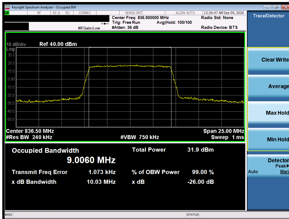
Plot 7-5. Occupied Bandwidth Plot (LTE Band 26/5 - 10MHz 16-QAM - Full RB Configuration)
