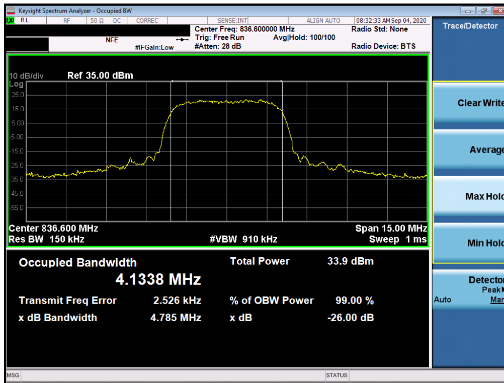
Plot 7-18. Occupied Bandwidth Plot (WCDMA, Ch. 4183)
