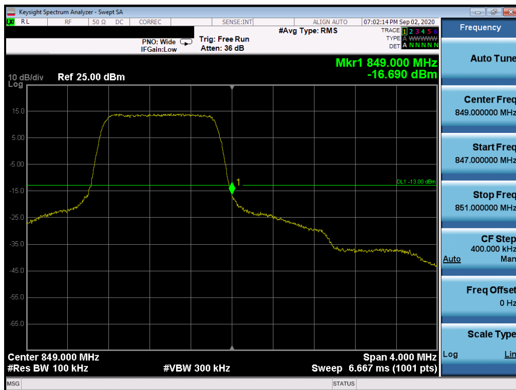
Plot 7-37. Upper Band Edge Plot (LTE Band 26/5 – 1.4MHz QPSK – Full RB Configuration)
