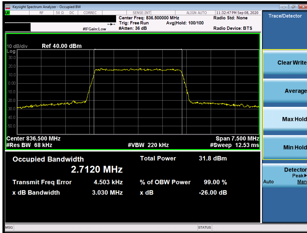
Plot 7-11. Occupied Bandwidth Plot (LTE Band 26/5 - 3MHz 16-QAM - Full RB Configuration)
