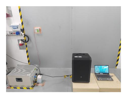
Set-up for Radiated Emission (RE), Below 1GHz
