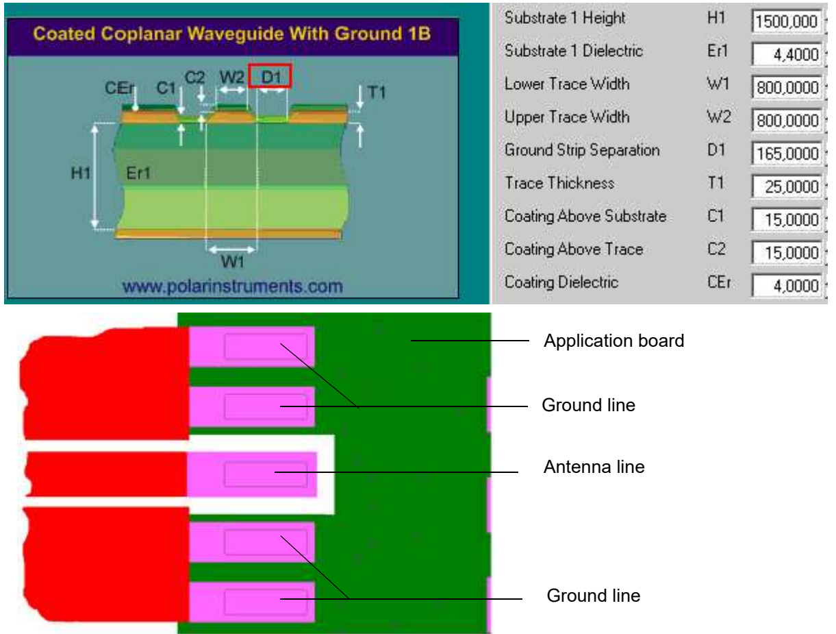
Figure 27: Micro-Stripline on 1.5mm Standard FR4 PCB - example 1
