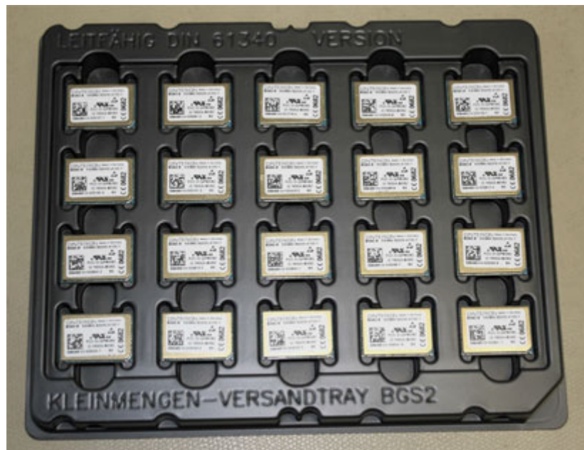
Figure 67: Tray to ship odd module amounts
