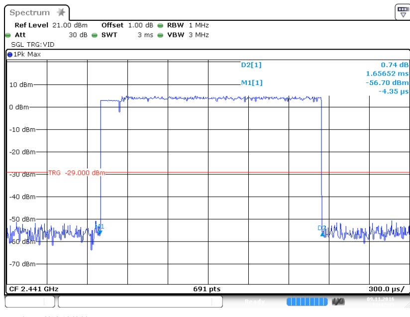
**Pulse time, High Channel, DH3**
