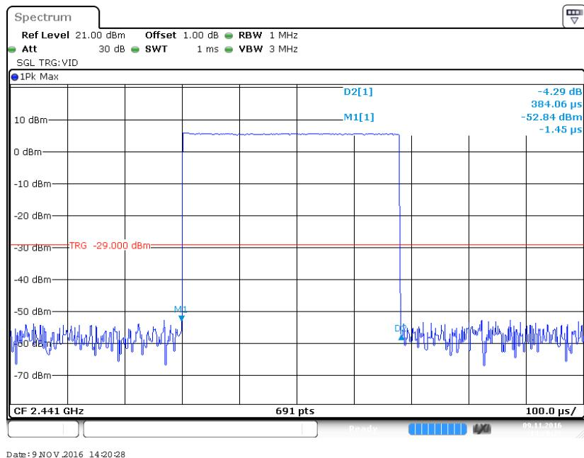
**Pulse time, High Channel, DH1**
