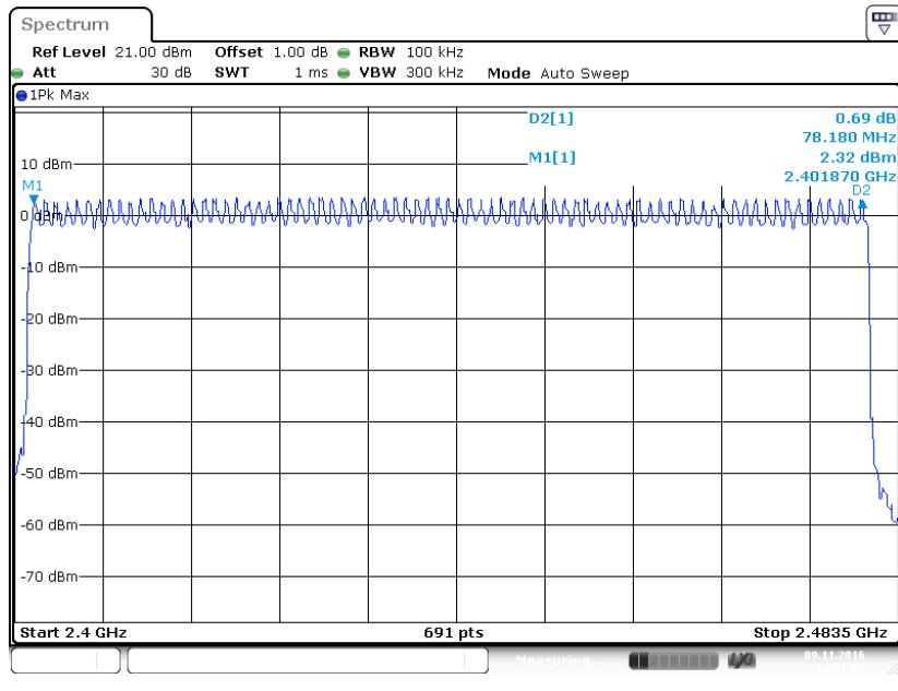
**EDR (8DPSK): Number of Hopping Channels**
