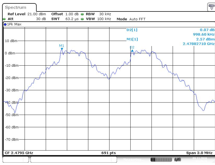
**EDR ( $\pi/4$ -DQPSK): Low Channel**
