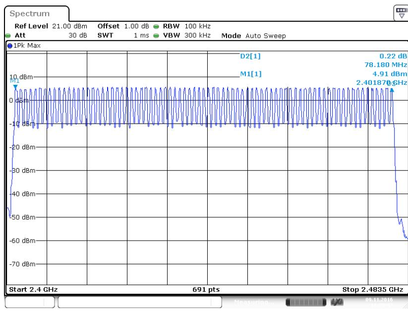
**EDR ( $\pi/4$ -DQPSK): Number of Hopping Channels**
