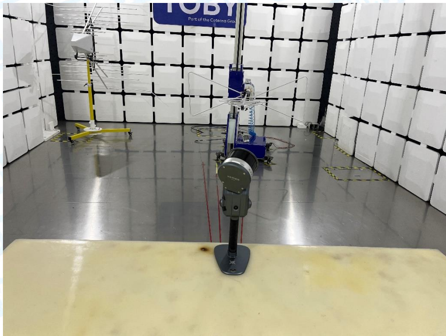
Photo of Setup for Radiated Emission (30MHz~1GHz)
