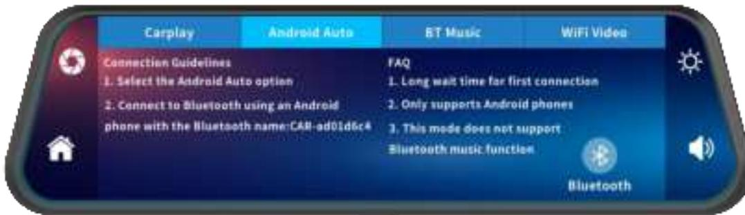
As shown in the figure above, click the [Android Auto] button to enter the Android Auto mode. First connection: click the [Bluetooth Management] management option on this interface, connect the Bluetooth with your phone, and then start the application;
