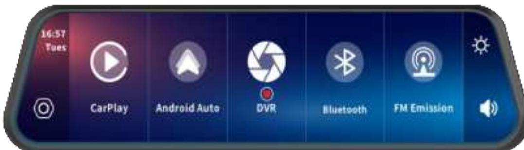
As shown in the figure above, the camera image will not be displayed on the main page. You need to click the [Dash Cam] button to view the camera image. When a card is inserted, the system automatically enters the recording mode. When recording, the red dot in the [Dash Cam] button will flash.
