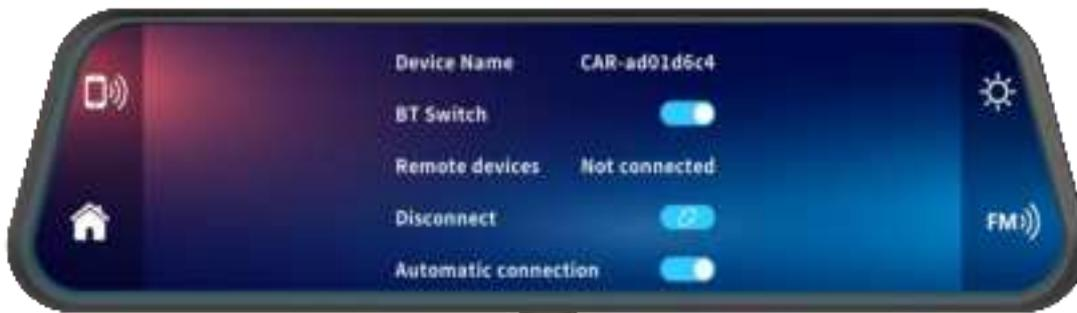
As shown in the picture above, click the [Bluetooth] button. After entering the Bluetooth interface, you need to turn on the switch button to turn on the device.
