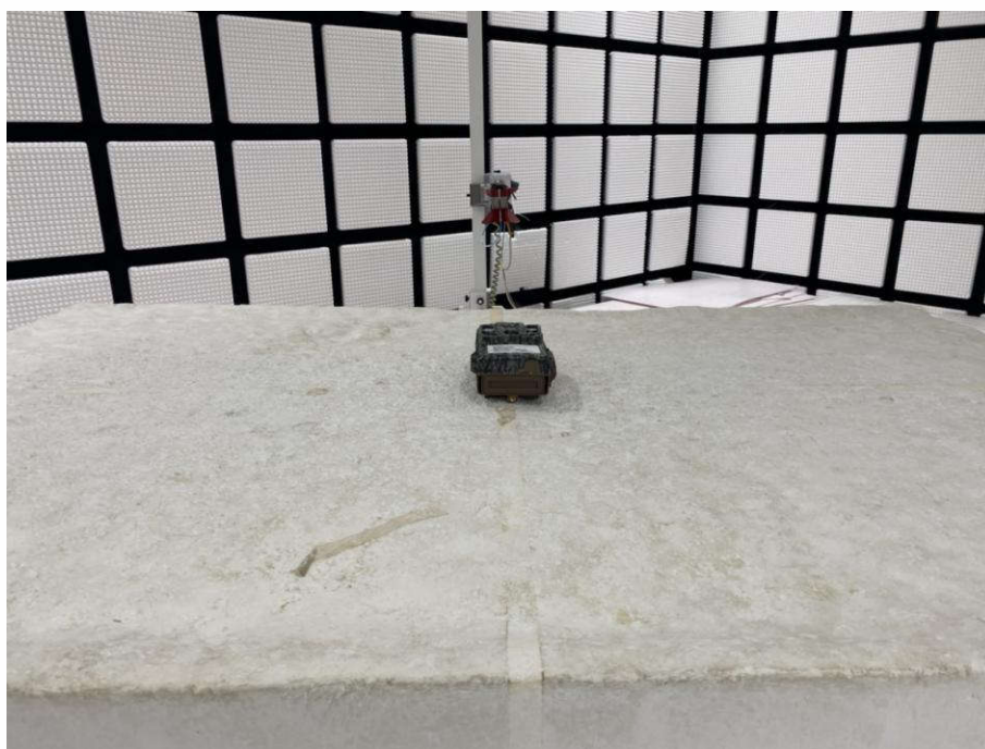
Radiated spurious emission Test Setup-2(Above 1GHz)
