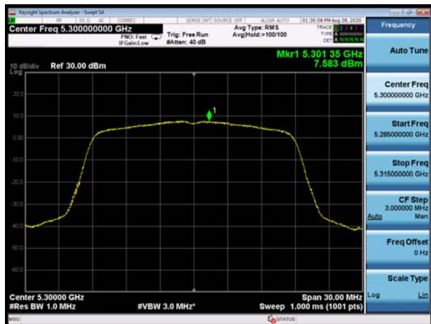
U-NII-2A, 802.11ac VHT20, Channel No.: 60
