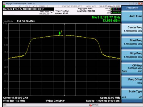
U-NII-1, 802.11ac VHT20, Channel No.: 40
