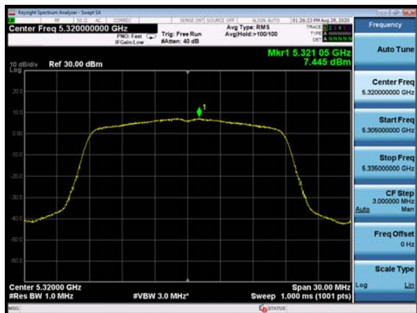
U-NII-2A, 802.11ac VHT20, Channel No.: 52
