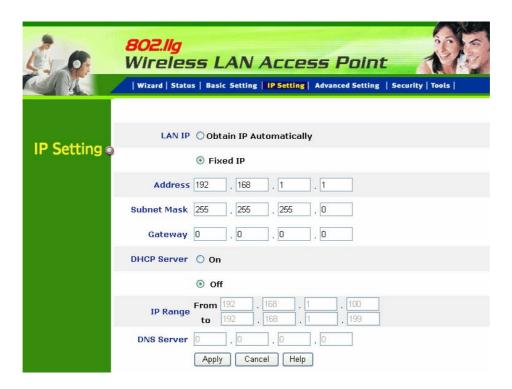
The default IP address of this access point is 192.168.1.1 with the subnet mask of 255.255.255.0. User can type in other values for IP Address, Subnet Mask and Gateway and click "**Apply**" button for the changes to be effective.
