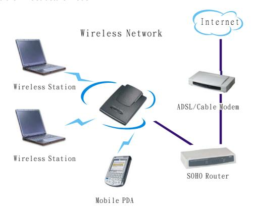
In order to setup an Infrastructure of a wireless network such as the example shown above, user will need the following:
