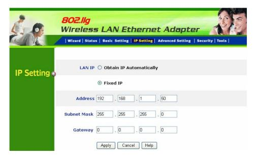
The default IP address of the Pocket Access Point in **Clint mode** is **192.168.1.50** with the subnet mask of 255.255.255.0. User can type in other values for IP Address, Subnet Mask and Gateway and click "**Apply**" button for the changes to be effective.
