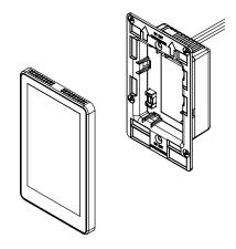
Thermostats should be installed after texture and paint. Each thermostat will be snapped into a pre-wired J-Box (at least 18 cu. inches). Once the Warmboard thermostats are powered up, they communicate wirelessly, so now additional wiring is required.
