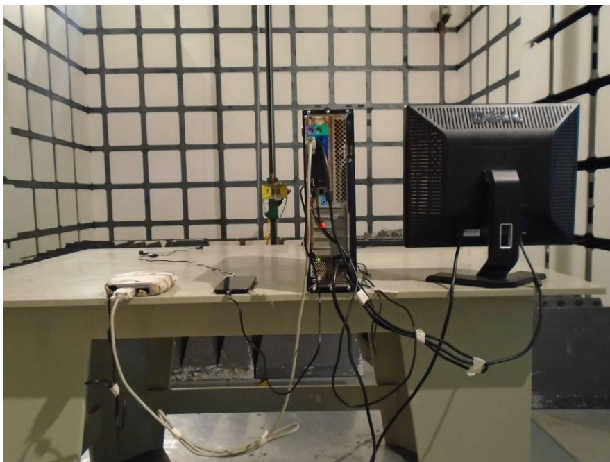
Radiated Emissions – Rear View (Above 1 GHz)
