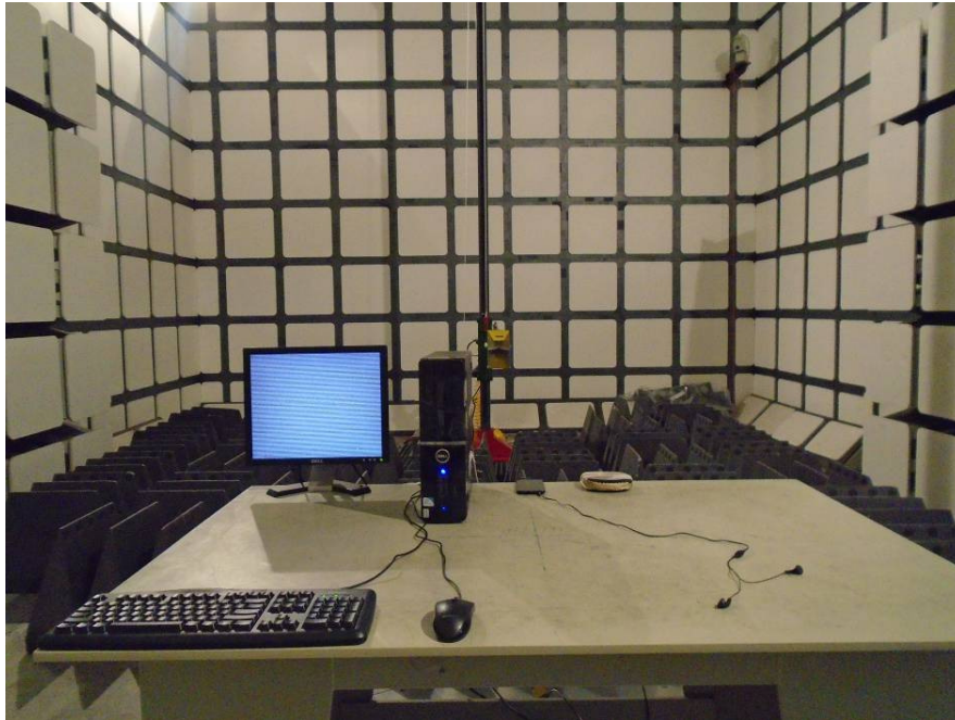
Radiated Emissions – Front View (Above 1 GHz)
