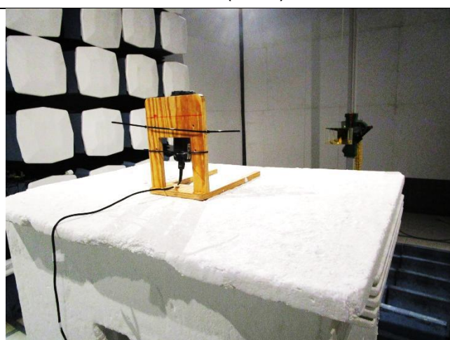
Radiated Emissions (>1GHz) – Rear View
