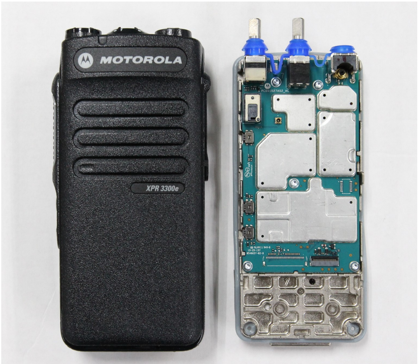
RF board with chassis and housing for Non Keypad model (front side)
