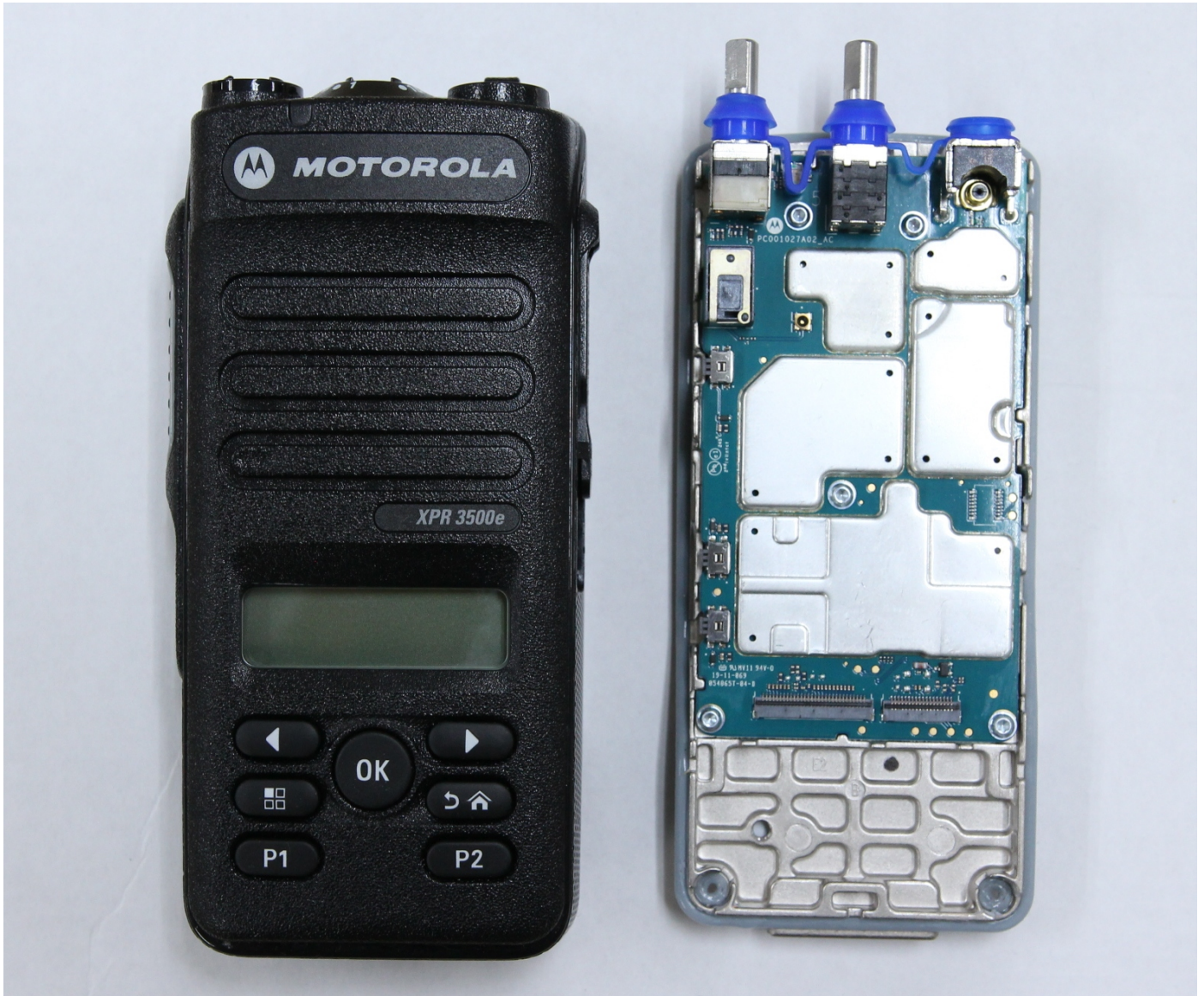
RF board with chassis and housing for Display and Limited Keypad model (front side)
