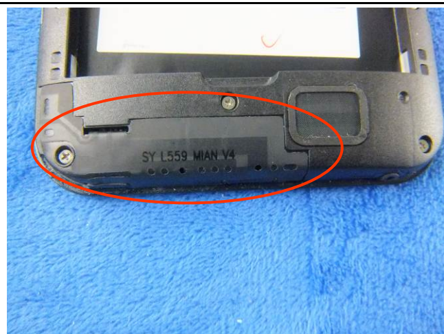
GSM/PCS/UMTS-FDD Antenna View
