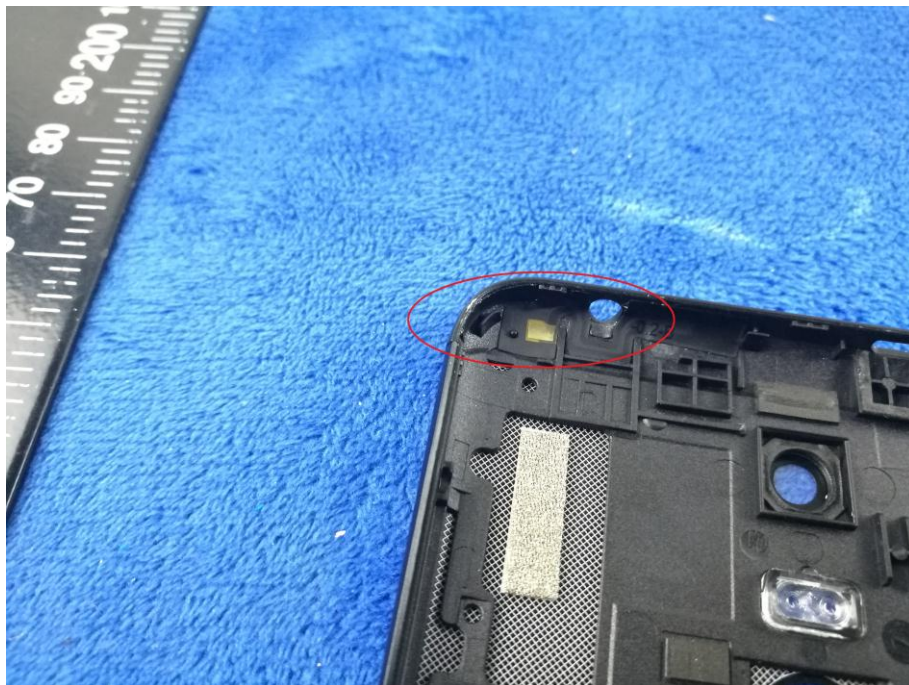
WIFI/BT/BLE/GPS - Antenna View
