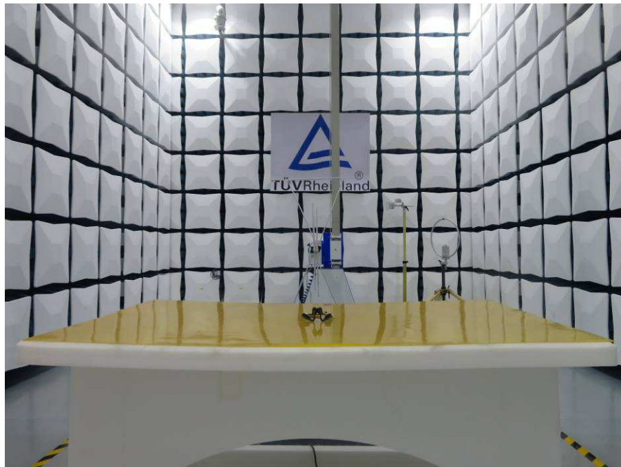
Photograph 1: Set-up for Radiated Spurious Emission, Below 1GHz
