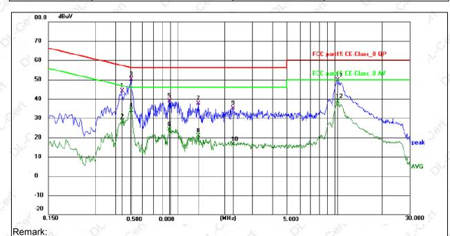
Margin = Limit – Level, Correct Factor = Cable lose + LISN insertion loss, Level= Reading + Correct factor
