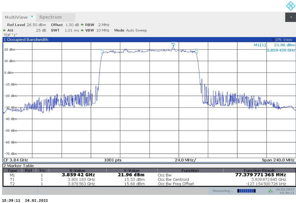
**n77H,80MHz Bandwidth,DFT-s-QPSK (99% BW)**
