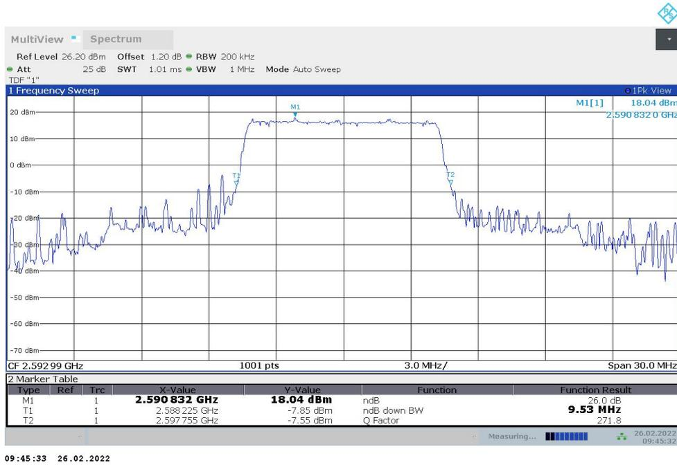
n41,10MHz Bandwidth,DFT-s-QPSK (-26dBc BW)
