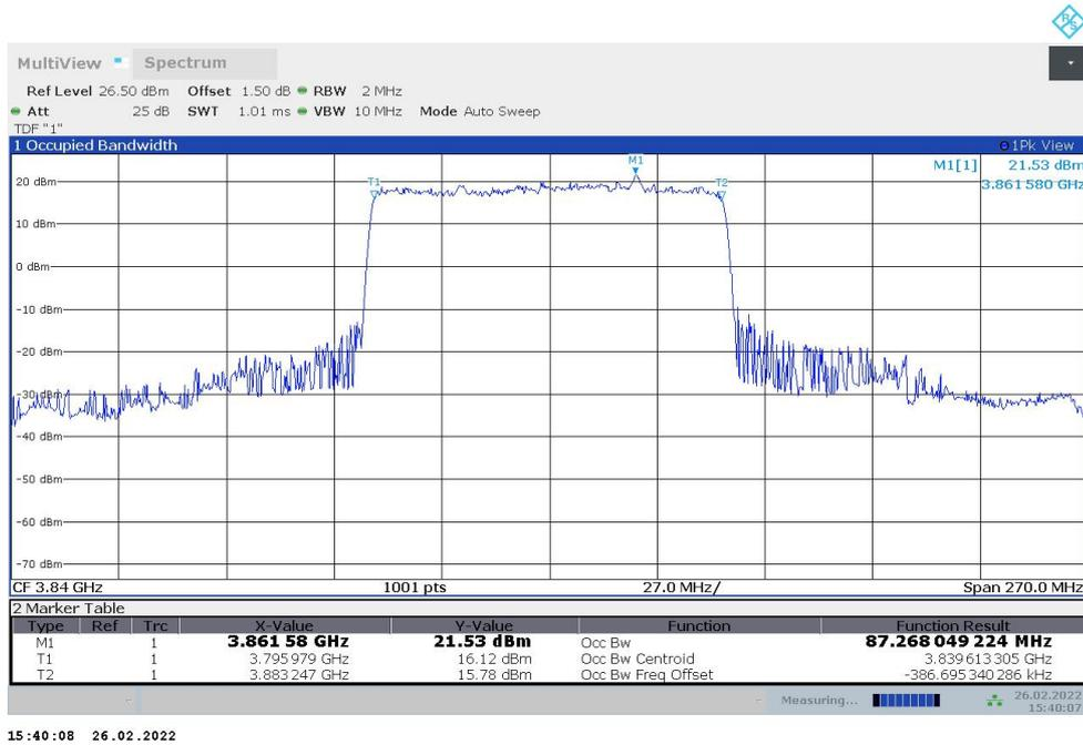
**n77H,90MHz Bandwidth,DFT-s-QPSK (99% BW)**
