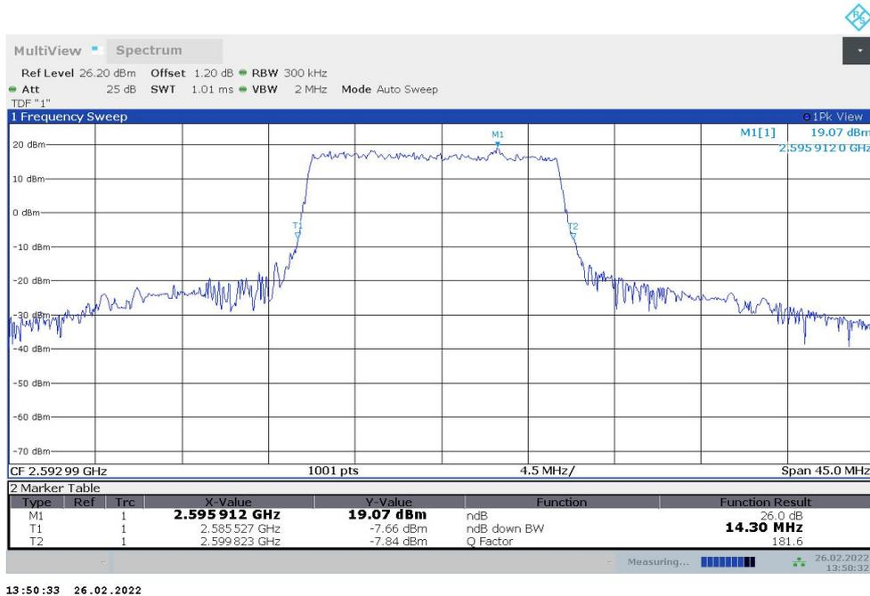
**n41,15MHz Bandwidth,DFT-s-QPSK (-26dBc BW)**
