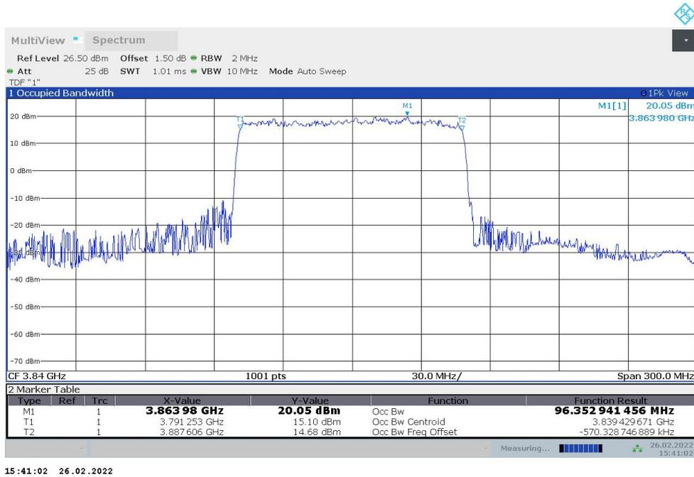
**n77H,100MHz Bandwidth,DFT-s-QPSK (99% BW)**
