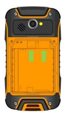
3. First match the lower part of the battery with the mobile phone metal part in the direction of Arrow 1 and then press the battery into the battery slot in the direction of Arrow 2.
