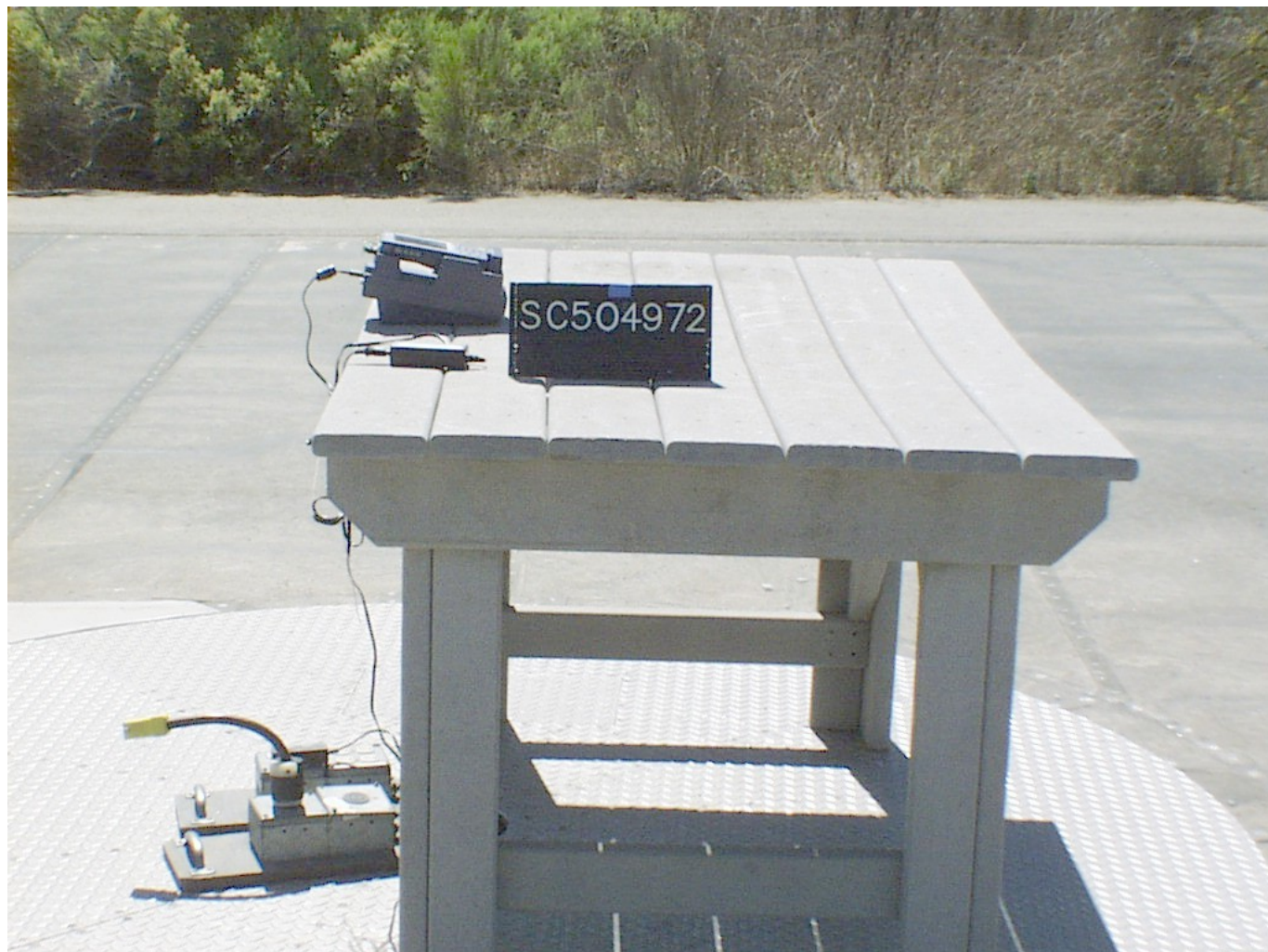
Photograph of Test Setup: Radiated Emissions
