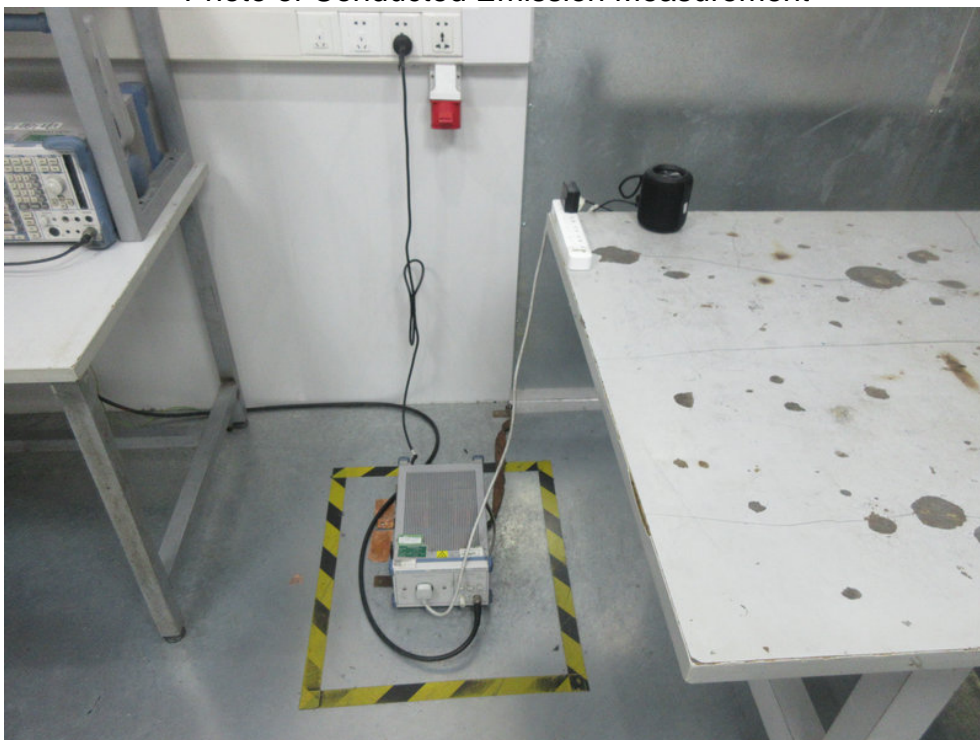
FCC ID: 2AL7B-OZE100 Photo of Conducted Emission Measurement
