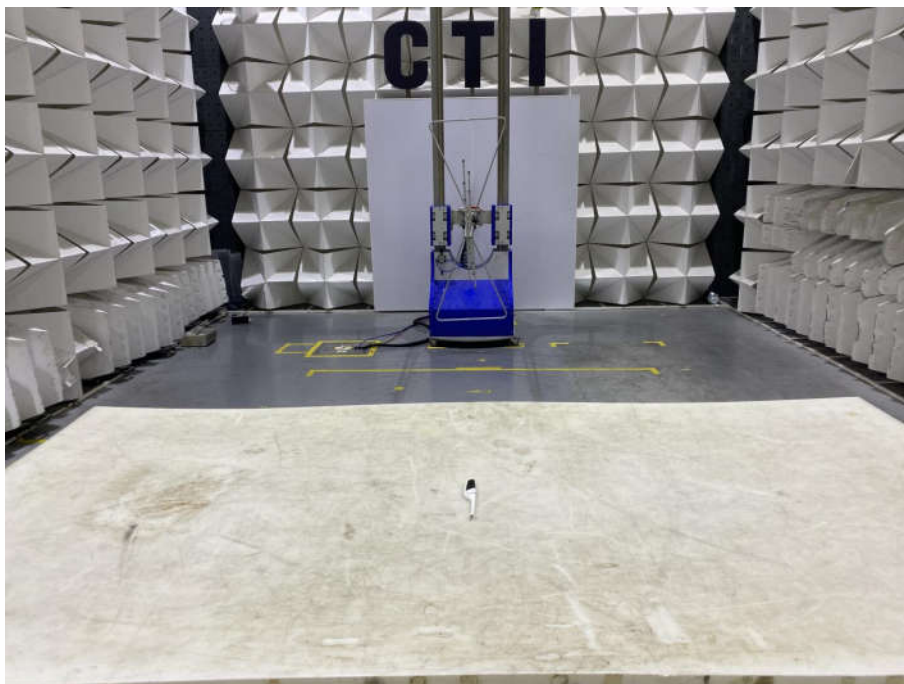
Radiated spurious emission Test Setup-2(Below 1GHz)
