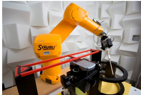
Figure 4-3 SPEAG Robotic System
