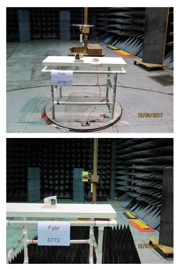
The EUT was taped to a foam stand in order to change the axis of rotation.
