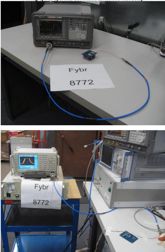
Photograph of Spurious Conducted Emissions Test Setup
