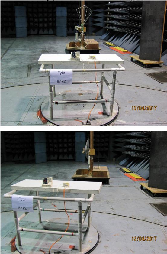
Photographs of Radiated Emissions Test Setup
