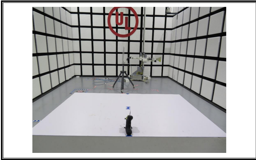
RADIATED RF MEASUREMENT SETUP (Below 30MHz – Z axis)
