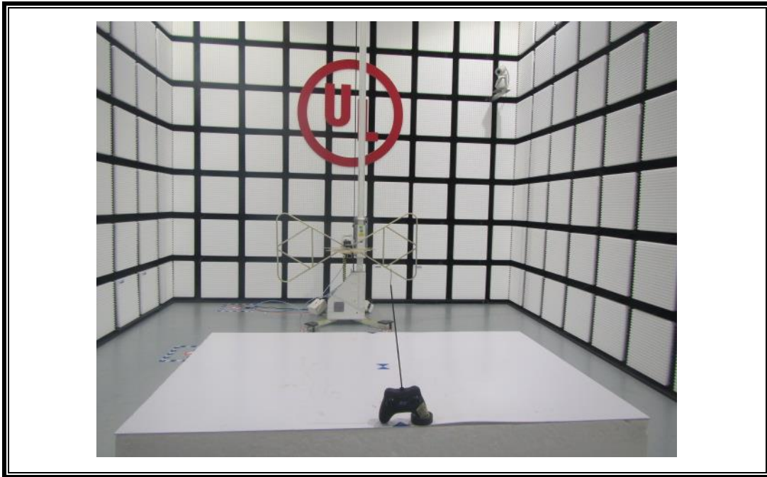
RADIATED RF MEASUREMENT SETUP (30MHz ~ 1 GHz)
