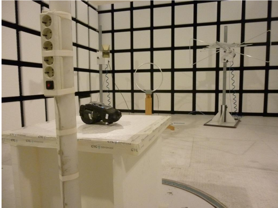
Photo 9: EUT at the anechoic chamber, magnetic loop antenna test setup
