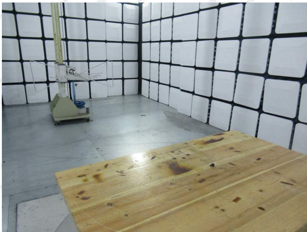
Photo of Radiation Emission Test
