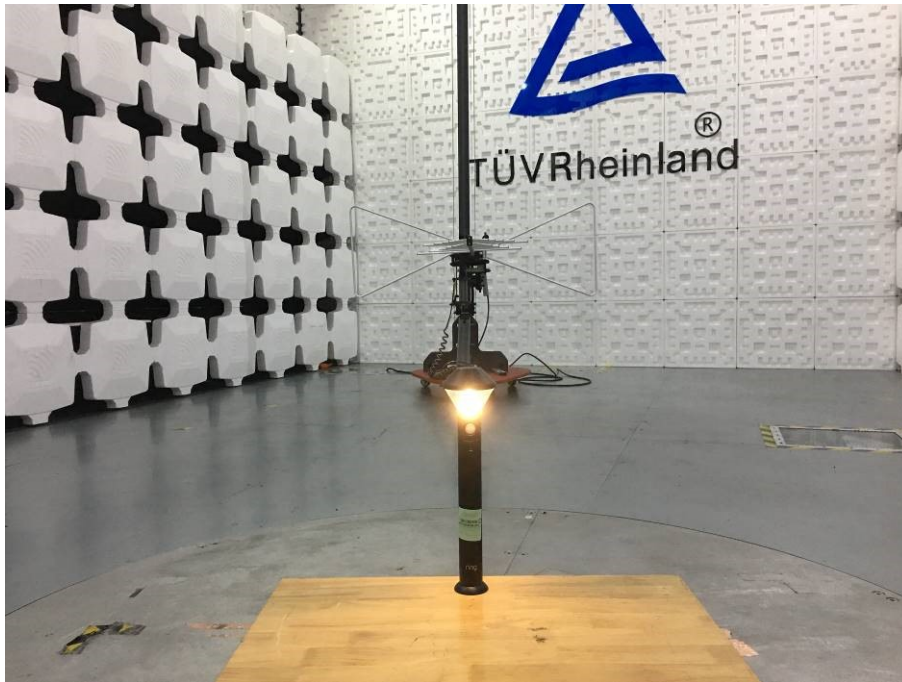
Photograph 3: Set-up for Radiated Emission, Below 1GHz
