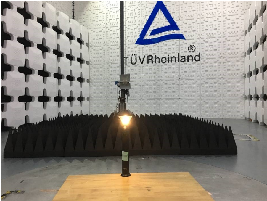
Photograph 4: Set-up for Radiated Emission, Above 1GHz
