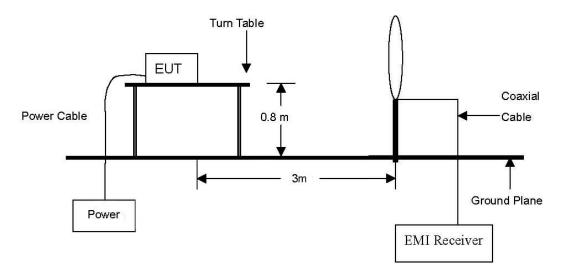
The diagram below shows the test setup that is utilized to make the measurements for emission from 30  $\,\mathrm{Mb}$  to 1  $\,\mathrm{Ghz}$  emissions.
