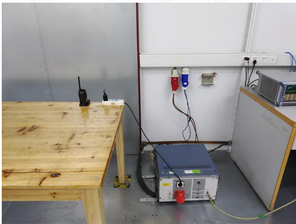
RADIATED EMISSION TEST SETUP-BELOW 1GHZ
