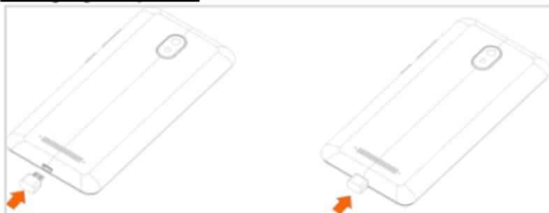
Insert micro USB end of the charging cable into the charging port of your phone. Plug the charger into a wall outlet or insert the regular end of the charging cable into any external USB port.
