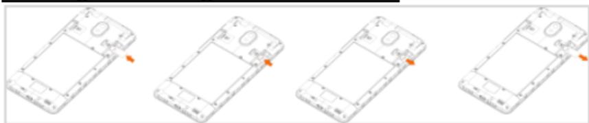
Place your SIM card into the Nano SIM compartment above with gold contacts facing down. Ensure SIM is correctly inserted. To remove SIM card, push the top of SIM card from opening and pull it out.
