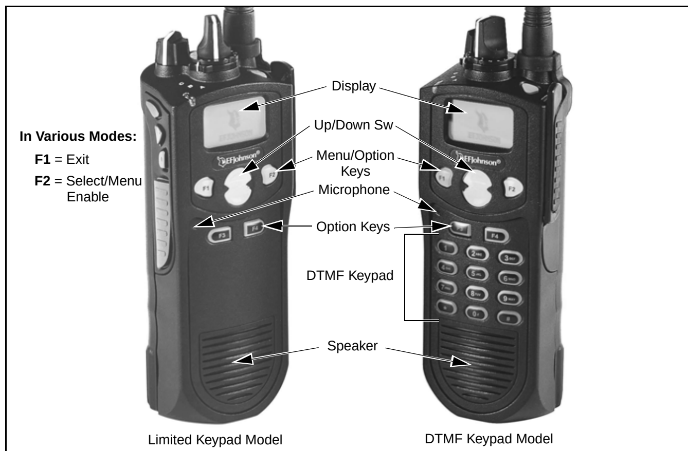
Figure 1-1 Front Panel Controls
