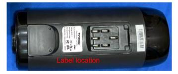
Permanent adhesive type is used to fix the label ,the label drawing isn't removed easily.
